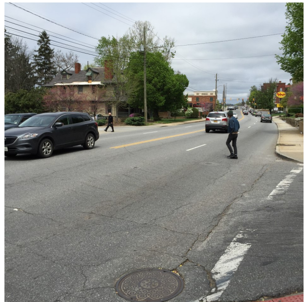
Pedestrian crossing Merrimon at Orange Street to reach a bus stop. The nearest signalized crossing of Merrimon with a pedestrian signal and crosswalk is at Chestnut. That signal is 650 feet away and requires a 1,300 foot out-of-direction trip to reach the other side. That out-of-direction trip could take 6 minutes of walking time, not counting delay in waiting for the WALK signal to cross Merrimon at Chestnut.
