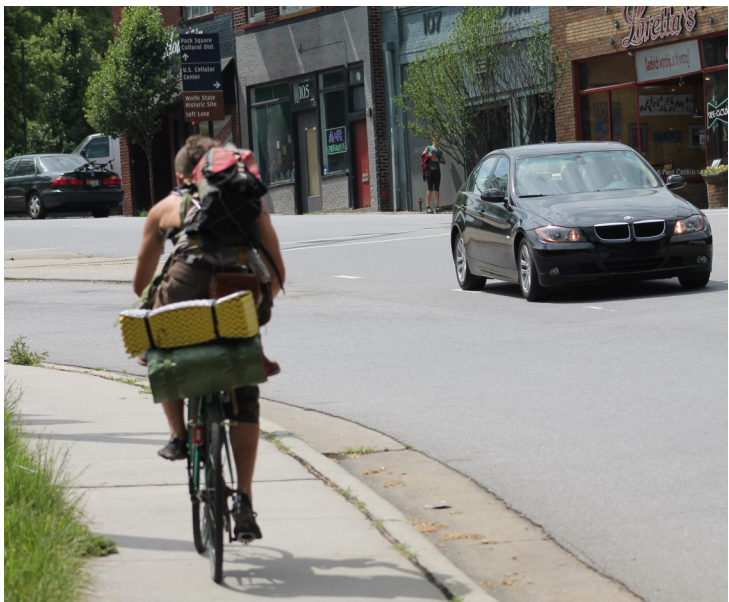
Figure 31: Bicyclist Using Sidewalk with 3.5 feet of Effective Width
