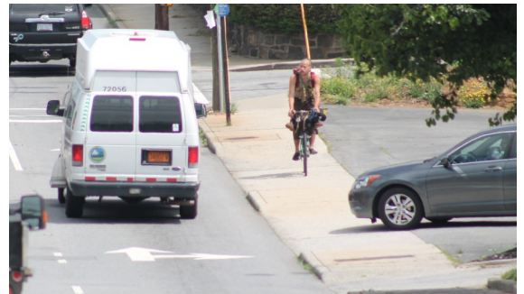
Driveway crossings have excessive cross slopes that can pitch wheelchair users into the street.
